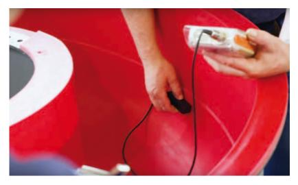
The thickness of the new wear lining is measured and documented
