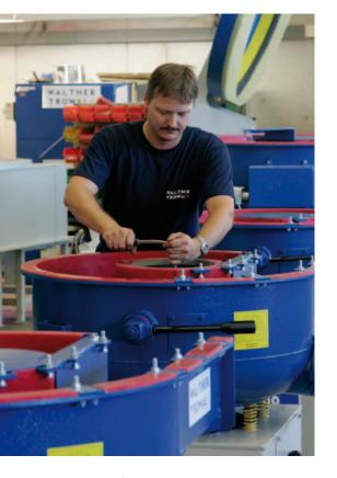
Refurbished work bowls in the final assembly stage.
